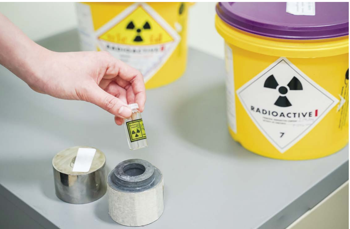
Open lead box of Iodine 131 (I-131) // Radioactive isotopes used for hyperthyroidism treatment // image supplied by Shutterstock
